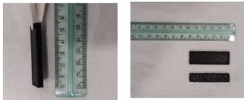
3D-printed specimens (10 x 50 x 2 mm)
