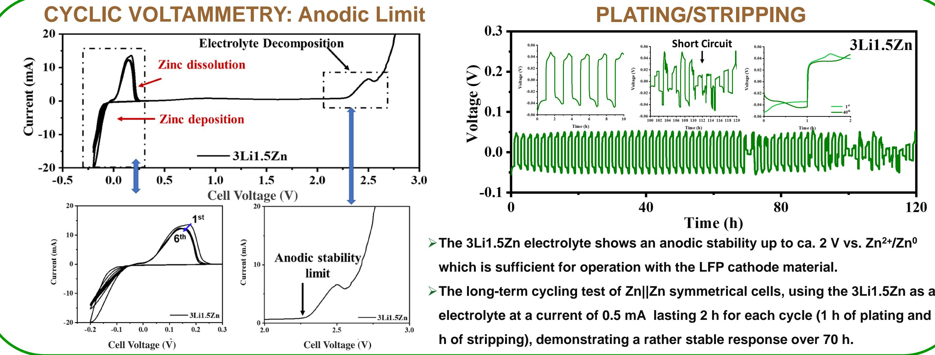
$\succ$  The long-term cycling test of Zn||Zn symmetrical cells, using the 3Li1.5Zn as an
