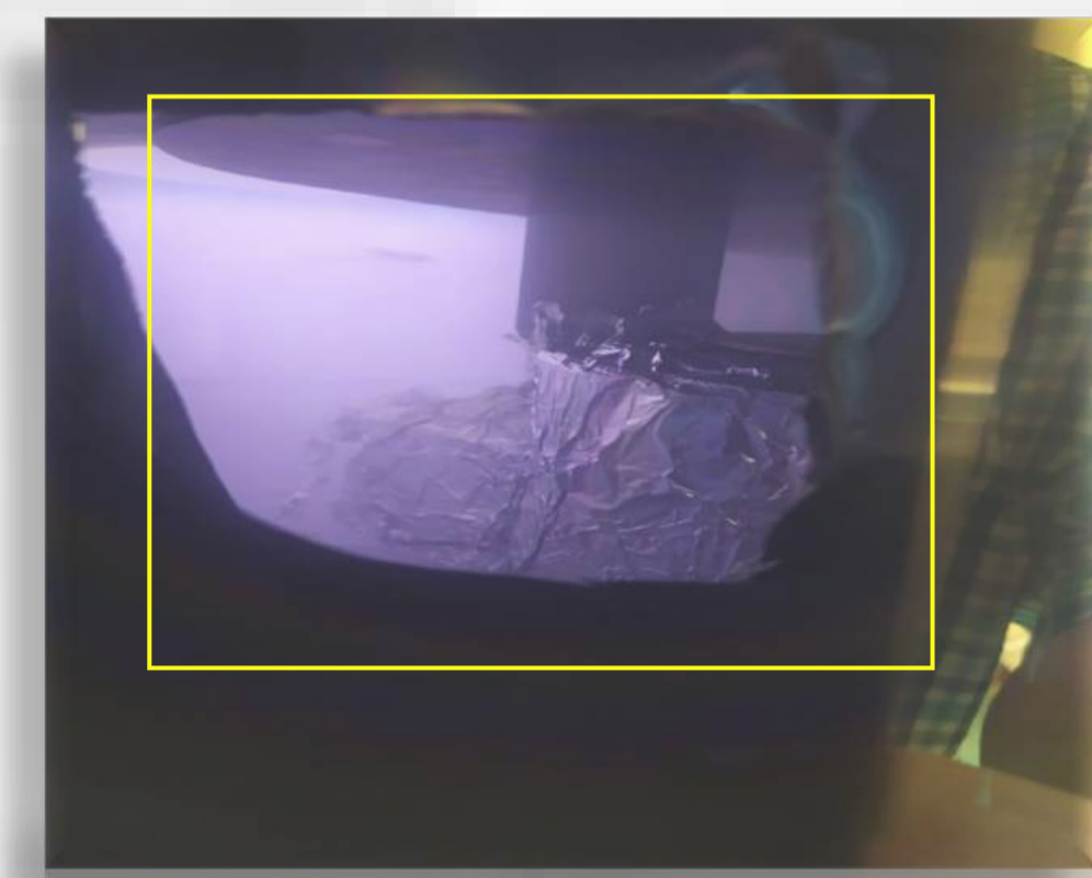
Figure 3. Plasma generated during deposition from the Sm doped ceria target.
