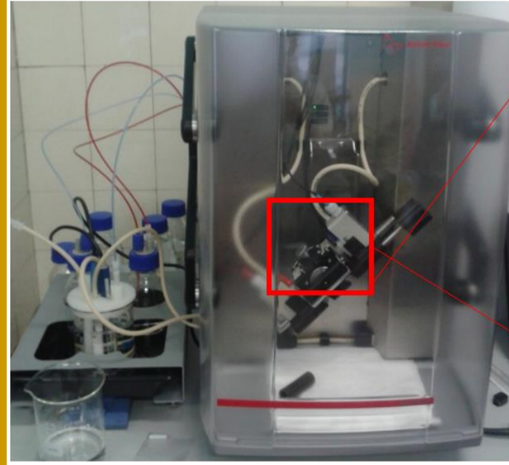
Figure 1: Electrokinetic Analyzer for the determination of zeta potential and test configurations
