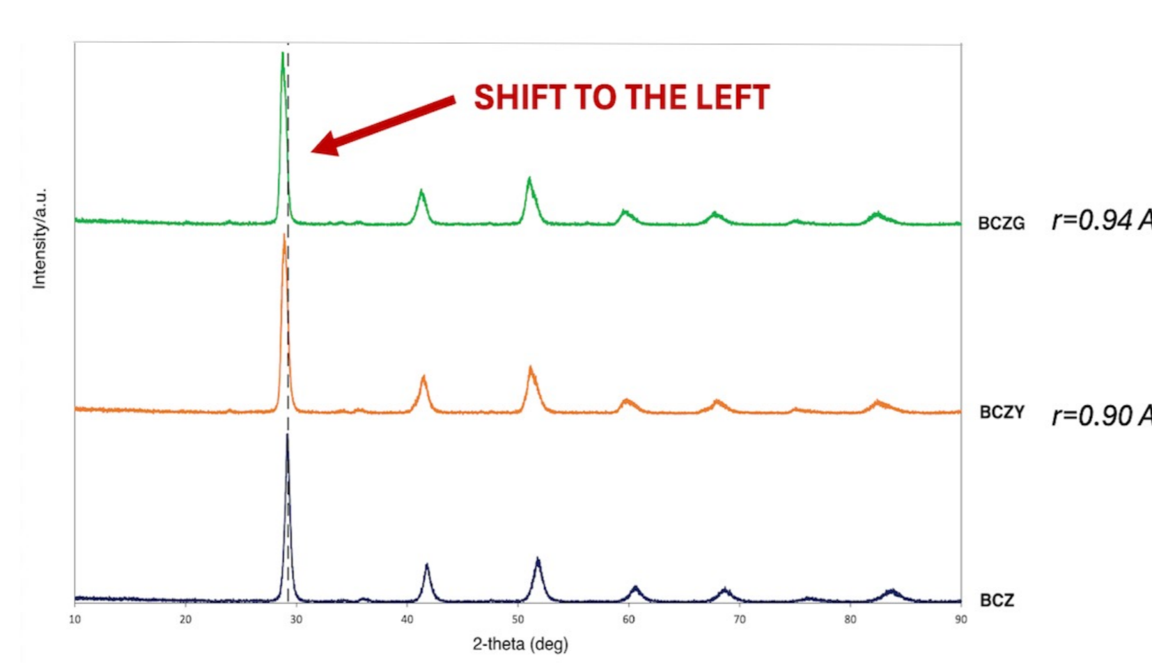
The XRD spectra of BCZ, BCZY and BCZG show that by including the dopant in the structure the peaks shift to the left with the increase of the ionic radius and thus the lattice parameters. The crystalline structure change from cubic pm-3m for BCZ to orthorhombic Imma for BCZY and BCZG.
