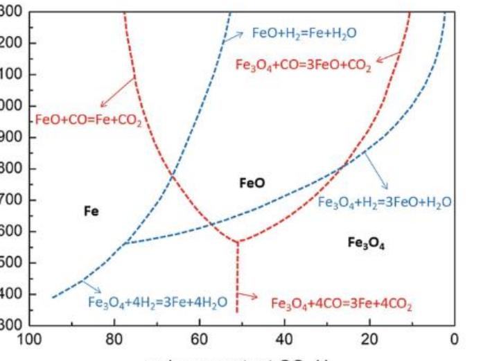
Fe-O-H<sub>2</sub> and Fe-O-C system including the Boudouard equilibrium for 1 bar and a carbon activity of 1.
